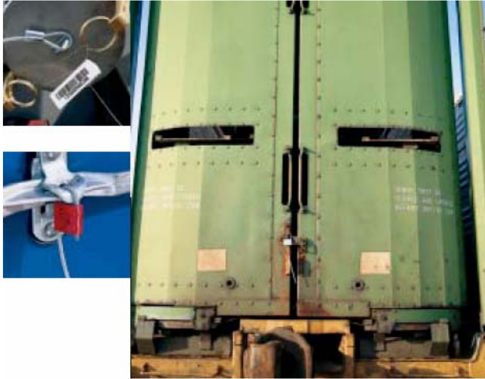
Figure 5-7. Cable Seal Applications.
